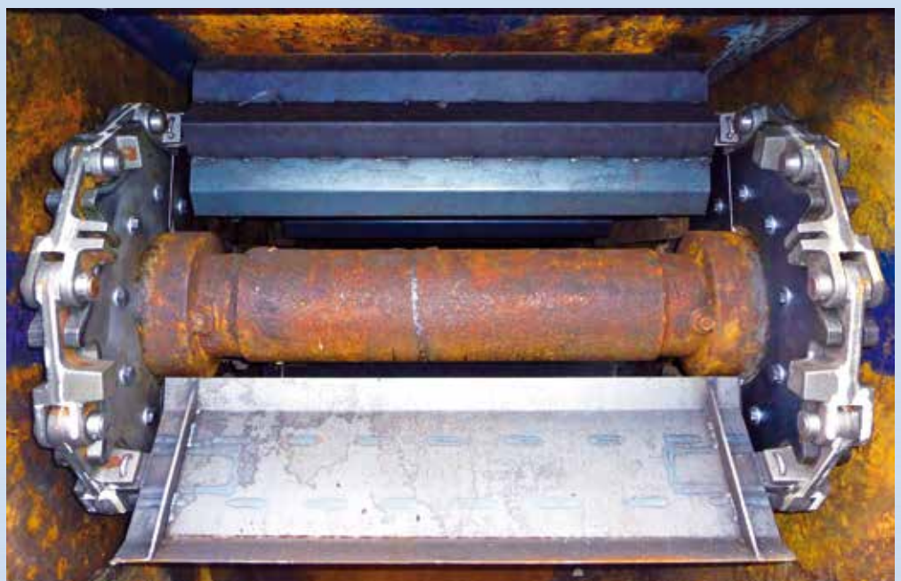
A new THIELE chain assembly fitted to a biomass conveyor
