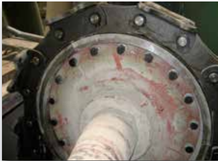
THIELE upgrade on an existing installation – optimum interaction between chain and chain wheel extends the operating life of the elevator.
